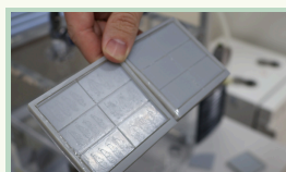
A microdevice made of polydimethylsiloxane (PDMS)
